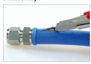
Place fitting and hose assembly in place and cut hose lengthwise from the blue cap approximately one inch.
